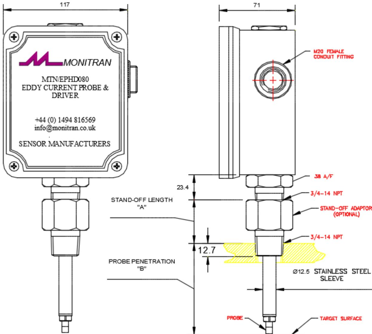
Note: it is recommended that for "A" plus "B" dimensions that are greater than 300mm an additional probe sleeve support is fitted at the probe end to stiffen the assembly and avoid resonance.
