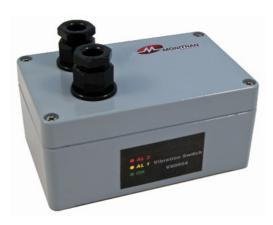
The MTVS0004 Vibration Switch offers a low cost, simple to install and operate solution to protect all sorts of rotating machinery; motors, pumps, fans, gearboxes etc. It's durable case with high IP rating is suitable for long life in harsh industrial environments. Measurements are made in velocity and compatible with ISO10816 Machine Vibration Severity Test.
