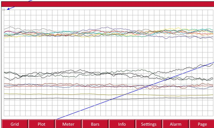
The plot screen displays channel values over time. The plot screen is 780 samples wide and displays 6.5 minutes of data @ 2Hz (default).
