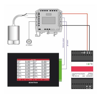
DIN rail-mounted single-sensor signal conditioning unit providing early warning of bearing and gear faults, imbalance, misalignment and looseness.
