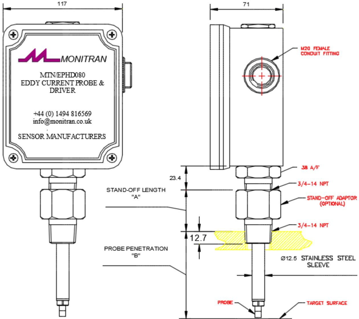
Note: it is recommended that for "A" plus "B" dimensions that are greater than 300mm an additional probe sleeve support is fitted at the probe end to stiffen the assembly and avoid resonance. (Additional support not supplied.)
