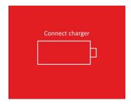
When the battery is level is low, a warning screen (see left) will display for 5 seconds and the unit will power off.
