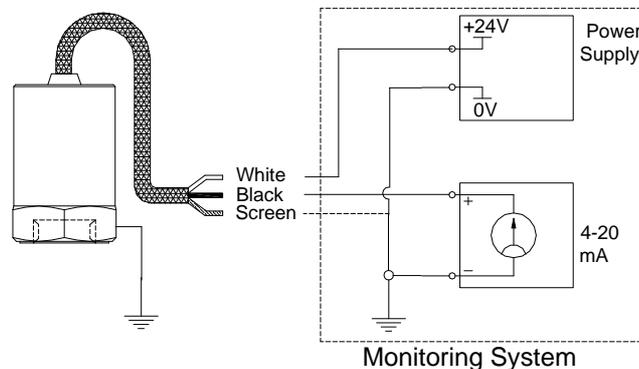
Fig 3: Control Circuit
