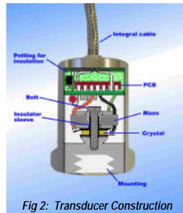
Fig 2: Transducer Construction
