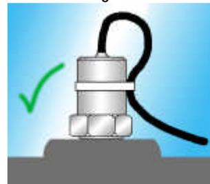
The cable should be fastened at suitable intervals to either a cable tray or convenient supports. This prevents accidental damage by personnel or moving machinery. To avoid excessive bending or axial thrust at the cable entry point or connector, loop the cable back and secure it to the transducer body with a tie-wrap. Fig 7
