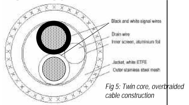
Fig 5: Twin core, overbraided cable construction
