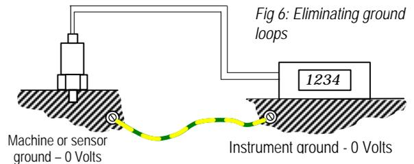
Fig 6: Eliminating ground loops
