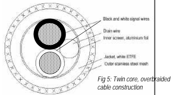
Fig 5: Twin core, overbraided cable construction
