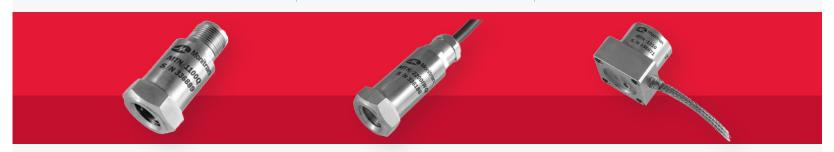
The MTN/1100R is a constant current accelerometer with an isolated AC output of 100mV (others available upon request) suitable for use in harsh radiation environments. Sealed to IP67, it has a frequency range of 2Hz to 10kHz and a temperature range of -55°C to 140°C.
