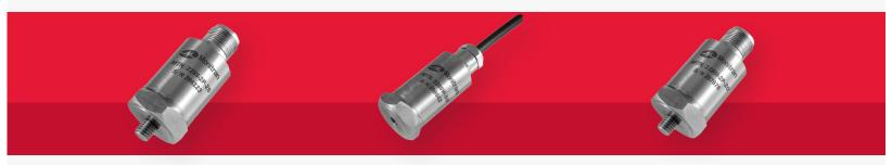
The MTN/2285-2P/4P/C is suitable for use in most industrial monitoring applications. Its output is proportional to velocity and it has a frequency range of 2Hz to 1kHz, a temperature range of -25°C to 90°C and is sealed to IP67.
