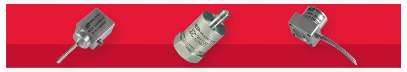
The MTN/1105SCE\* is constant current AC output accelerometer for vibration analysis at temperatures up to 250°C. It has a frequency range of 0.8Hz to 12kHz and a sensitivity of 100mV/g (others are available upon request).
