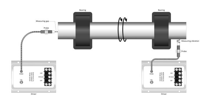
Eddy current displacement sensors are non-contact devices capable of high-resolution measurement of the position of a conductive target. The probe consists of a thermally stable plastic tip and when connected to the driver unit it produces a high frequency oscillation that induces eddy currents in the target material.
