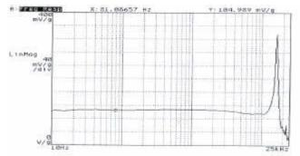
Fig 4: Typical Response Curve for MTN/1100
