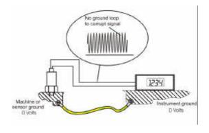
Fig 6: Eliminating ground loops
